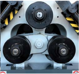
3 RULLI TRASCINATORI 3 FORMING ROLLS 3 WALZEN RETREATS
